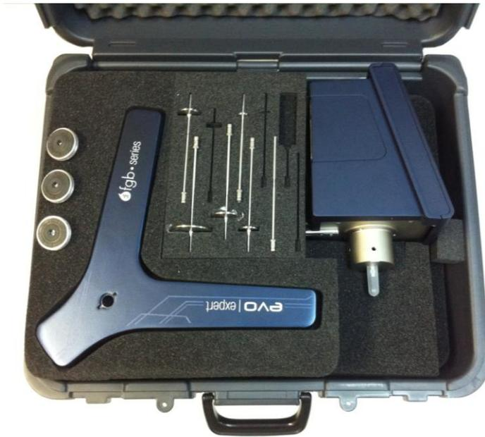
Fig 1. Viscometer in its carry-case
