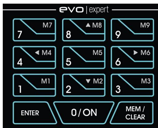
Fig. 6 The keyboard for the Evo Expert viscometer
