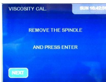
Remove the Spindle if it is connected to the viscometer and press 'ENTER'. Then, the viscometer will perform the Offset calibration, showing the following screen:
