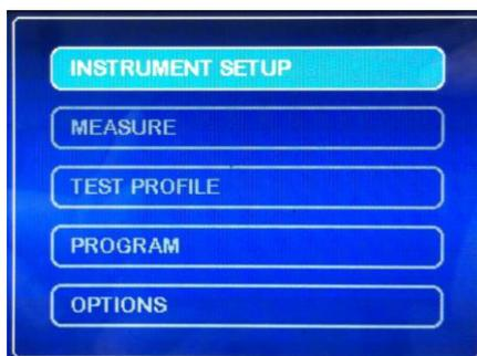
The menu can be navigated with the 'Δ' and '∇' keys. The current selection will be highlighted and by pressing 'ENTER' you will access to the selected submenu (for more information about each function in particular see the corresponding sections).
