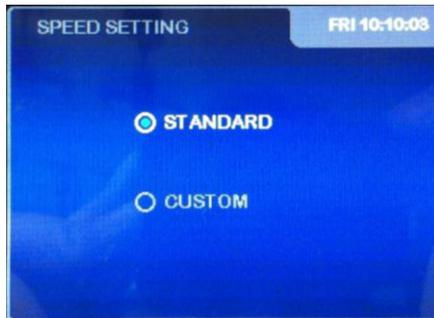
This is the 'SPEED SETTING' submenu screen. The Evo EXPERT series viscometer has a pre-set speed with a total of 56 RPMs (revolutions per minute) as well as speeds in which the RPMs can be set manually. In some cases, when the work speeds are repetitive, the user can personalize these speeds configuring a profile for the measurement.
