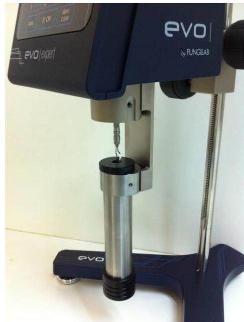
Fig.8: LCP Adapter assembled in viscometer
