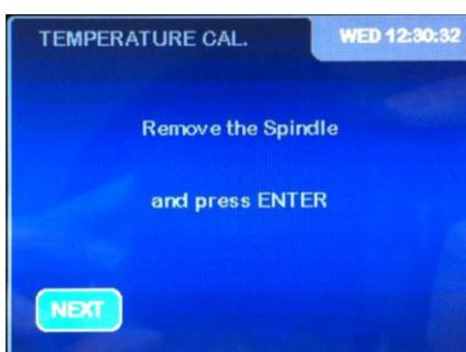
**VERY IMPORTANT:** The Test-run should be carried out without a spindle.
