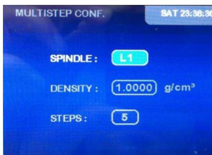
This screen shows the set's MULTISTEP program configuration. In this case, it shows that the L1 spindle is being used and that 5 steps are configured in the program. The 'SPINDLE' field appears highlighted by default. Use the 'Δ' and '▽' keys to choose the spindle and then press 'ENTER'.
