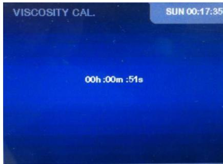
The spindle must already be submerged in the liquid once you confirm the start time. When the countdown gets to zero, the viscometer will start the calibrating sequence. While the equipment is calibrating, the following screen will appear (example):
