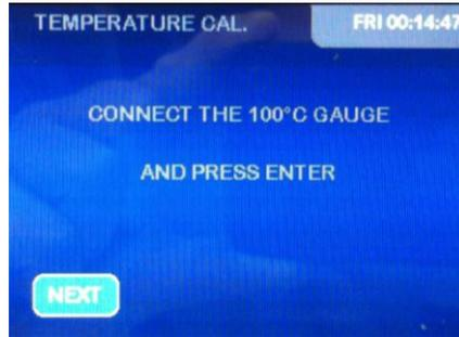
Now, you'll have to connect the PT100 simulator generating impedance equivalent to a 100°C PT100. With the gauge connected and hitting the 'ENTER' key, this screen will appear:
